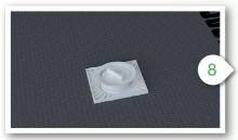
Fix the shower tray into position. With a spirit level, check that the edges of the tray are level. Also you should use waterproof tape to connect all joint and wall corners.
